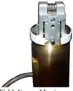
Weld Force Monitor: We packaged 2 load cells with preload in a device the size of a metered dose inhaler to aid set up of automated ultrasonic welders.
