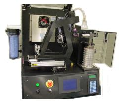
Automated Shaker Firer: We developed the enclosure and configured a 2-axis table, rotary shaking action and environmental controls for this automated testing station.
